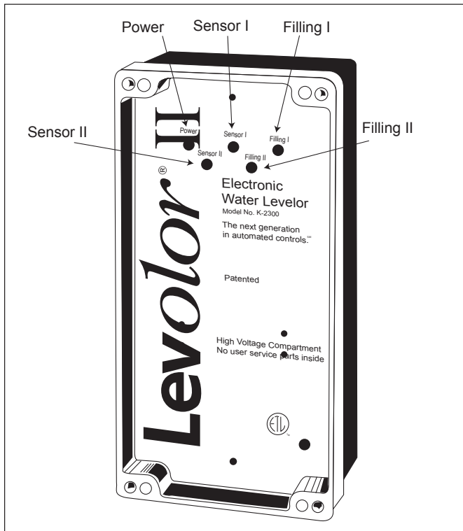
Figure 24. K-2300 Controller Lights
